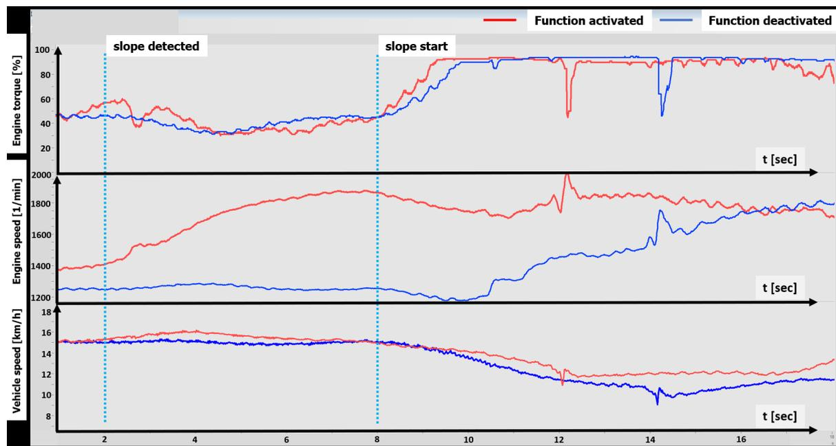
Figure 12: Representation of the uphill gradient recognition (© ZF Friedrichshafen AG)
