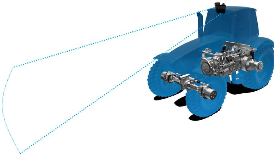
Figure 4: Assembly of radar on agricultural machinery (schematic view) (© ZF Friedrichshafen AG)
