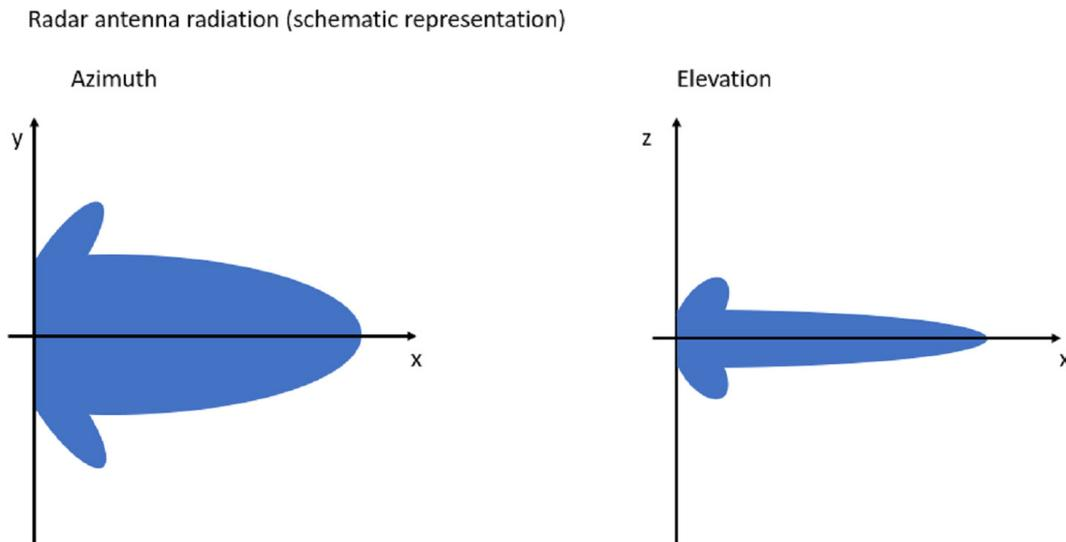
Figure 5: Radar cone (schematic representation) (© ZF Friedrichshafen AG)
