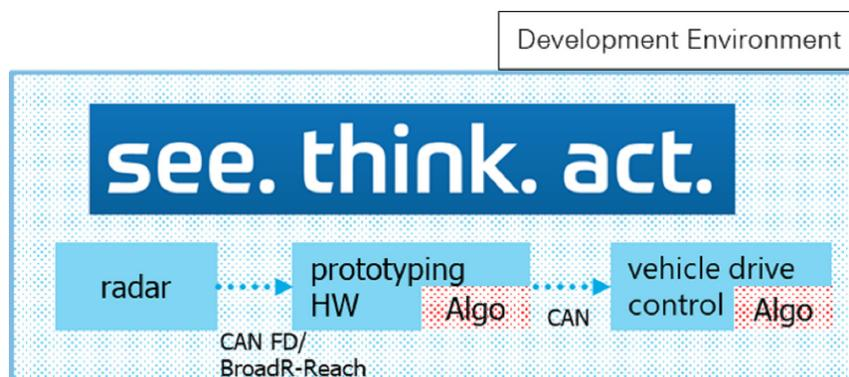
Figure 3: Embedding the algorithms in the development environment (© ZF Friedrichshafen AG)
