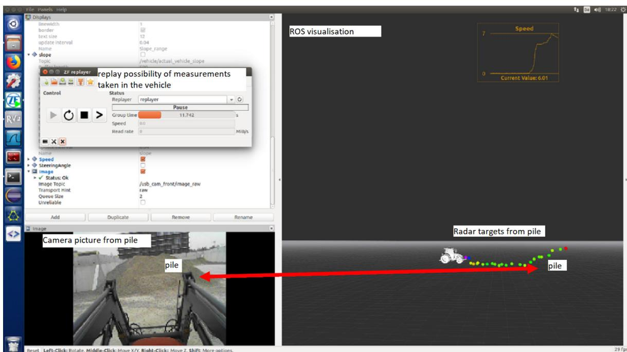
Figure 8: Visualization of the radar data in the ROS development environment (© ZF Friedrichshafen AG)
