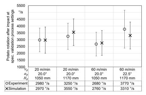
Figure 9: Comparison simulation and experiment of potato tuber angular velocity after impact
