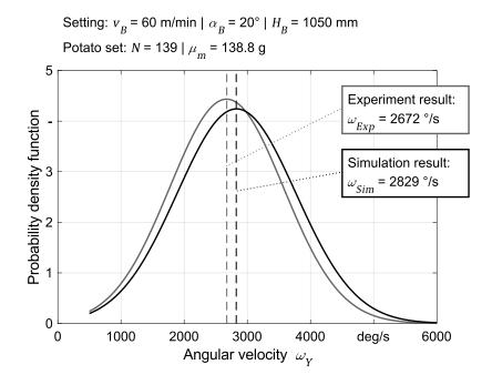
Figure 8: Distribution of angular velocity of potato tubers after impact for simulation and experiment
