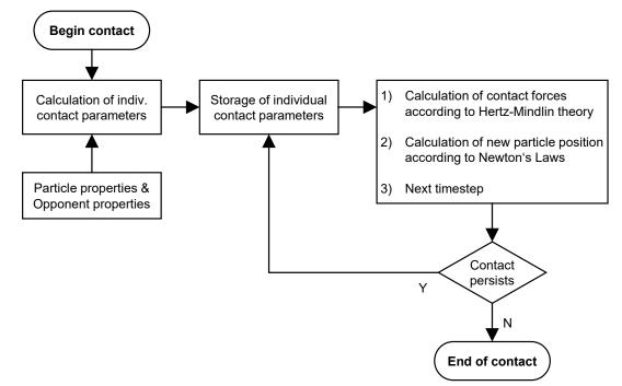
Figure 3: Flow chart of adaptable contact model in the environment of DEM Software EDEM
