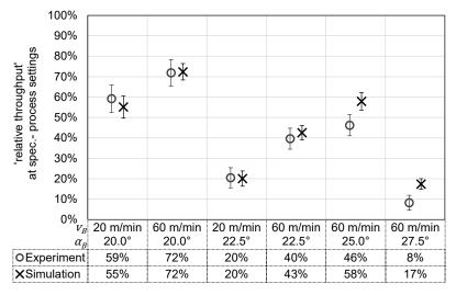
Figure 7: Comparison of 'relative throughput' between simulation and experiment
