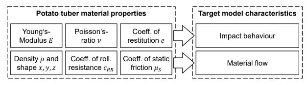
Figure 4: Parameter of potato particle model and target model characteristics
