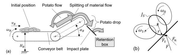
Figure 5: Concept of the validation rig and process (a) with a detailed view (b) on the impact of potato tubers and the angular velocity
