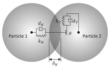
Figure 2: Viscoelastic contact model of two interacting spheres
