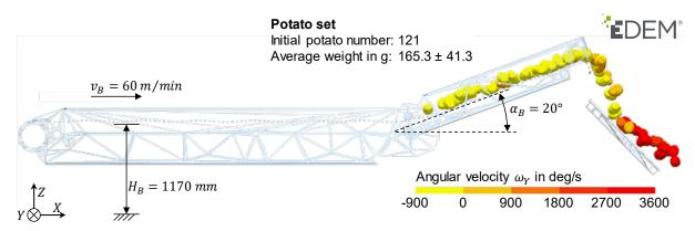
Figure 6: Lateral view of the simulation model with particle colored based on the angular velocity in Y-axis
