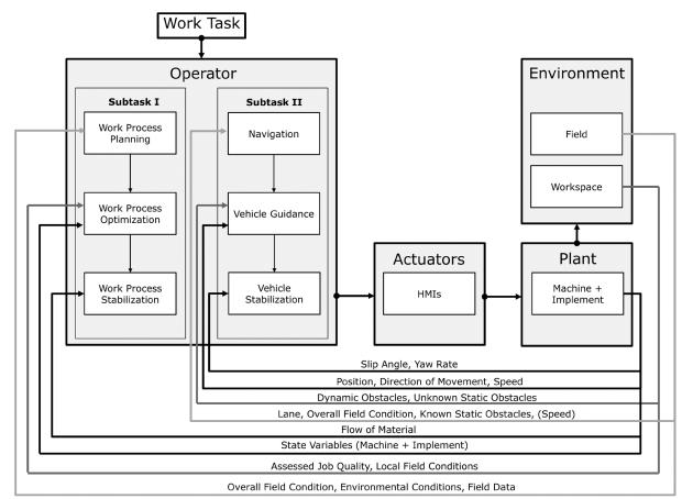
Figure 1: 3-level model describing the work task for the operator of a tractor-implement combination
