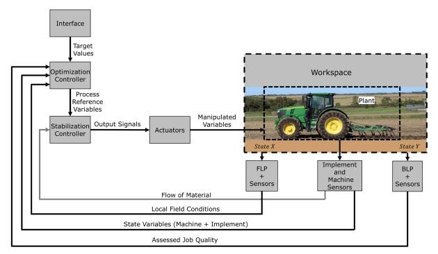
Figure 2: Visualization of the subtask "Monitoring and Controlling the Work Process" translated into an overall technological approach for tillage
