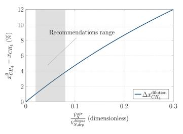
Figure 4: Theoretical process of methane concentration reduction through air injection. This example is calculated for  $x_{CH4}^0$  = 52 % according to Equation 4. On the left side of the recommendation range, the reduction represents approx. 1 percent and, on the right border, approx. 4 percent.
