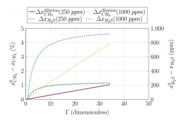
Figure 3: The process of H<sub>2</sub>S concentration reduction through biological desulfurisation with the model values from our trials. Additionally applied here is the theoretical maximum reduction of the methane concentration as a result of air injection. This example was calculated for  $x_{CH4}^0 = 52\%$  and  $x_{H2S}^0 = 250$  ppm/1.000 ppm with Equation 5 as well as Equations 3 and 7.
