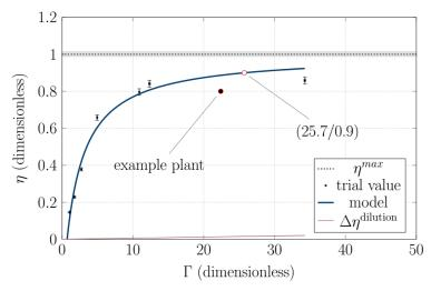
Figure 2: Process of the desulfurisation efficiency over the dosage of injected air. The upward H<sub>2</sub>S reduction trend progressively reduces as air flow increases. The possible maximum (i. e. absolute) desulfurisation takes place where  $\eta^{max} = 1$  statt.  $\Delta \eta^{dilution}$  is here determined for  $\chi^0_{H2S} = 250$  ppm ppm according to Equation 6. The positioning of the example plant is described in the text.
