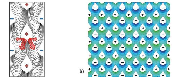
Figure 3: Simulated air flow distribution in the experimental dryer with horizontal configuration of the air ducts: (a) flow line presentation and (b) pressure distribution (static particulate bed; air flow rate of 465 m<sup>3</sup>/h), (+) inlet air and (-) outlet air ducts.
