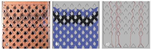
Figure 2: Particle movement in the test dryer: (a) experimental, (b) numerical and (c) particle trajectories
