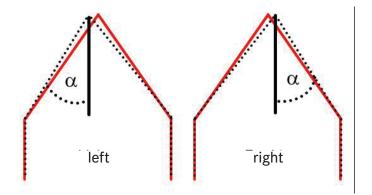
Figure 5: Geometric presentation and qualitative comparison of the original (red line) and the new devel-oped (dotted line) roof geometry
