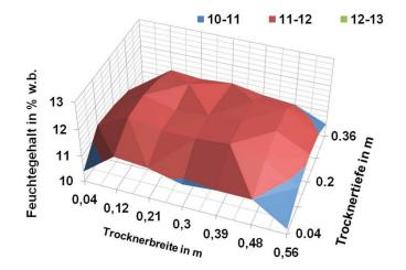
Figure 4: Average moisture content over the dryer cross section at outlet, measured in semi-technical scale, see Figure 1
