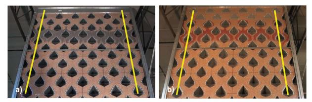
Figure 6: Experimentally measured particle flow profile for (a) conventional air ducts and (b) new developed air ducts (with altered roof angle in the vicinity of sidewalls) (© F. Weigler)
