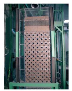
Figure 1: The geometry of the experimental dryer without air inlet and outlet duct hoods for process analysis of particle flow, airflow and the drying process (© F. Weigler)
