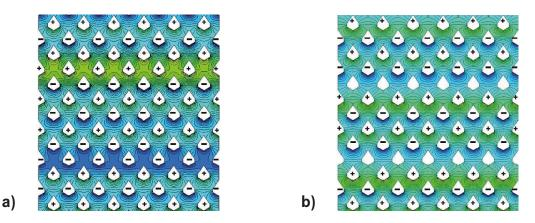
Figure 7: Pressure distribution in the MFD for (a) horizontal configuration of the air ducts with revolved sections and (b) the new design with a row of closed ducts per dryer section simulated with an air flow rate of  $465 \text{ m}^3/\text{h}$
