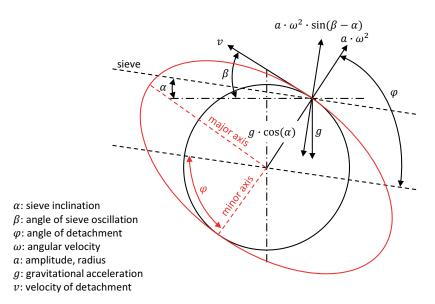
Figure 1: Dependency of the flight number *Fr* on the angle of detachment of the grain-MOG-mixture on a circular and an elliptical sieve movement (ROTHAUG et al. 2003)
