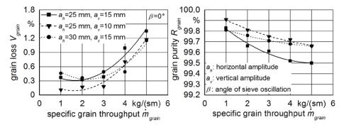
Figure 7: Comparison of the elliptical sieve movement with different parameter sets
