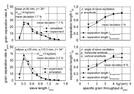
Figure 9: Comparison of the grain separation rate  $A_{grain}$  and the grain separation length  $l_{\theta0}$  of simulation and experiment for linear (BECKMANN et al. 2016) and elliptical sieve movements
