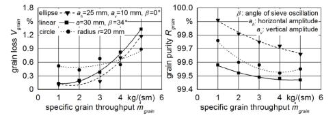
Figure 8: Comparison of the elliptical, circular and linear sieve movements
