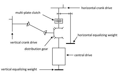
Figure 3: Drive of the sieve of the cleaning unit test rig (MEYER 2015)
