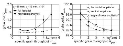
Figure 6: Comparison of grain loss and grain purity of a full factorial experimental series with the results from the regression analysis with a quadratic regression approach
