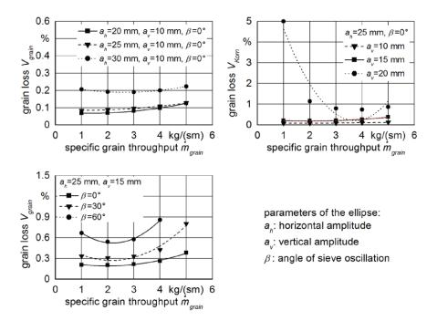
Figure 5: Influence of the horizontal and vertical amplitudes as well as the angle of oscillation on the grain loss based on a regression analysis with a quadratic regression approach
