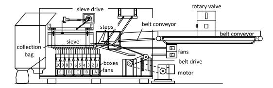
Figure 2: Combine cleaning unit test rig to investigate linear, circular and elliptical sieve movements (BECKMANN et al. 2016)
