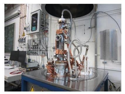
Figure 6: Heat exchanger under the high vacuum bell (© HAW Landshut)
