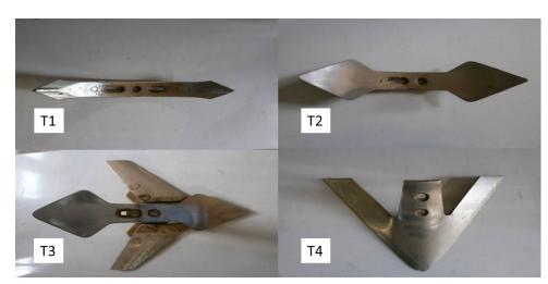
Figure 1: Standard single tines used in the experiment (© A. Al-Neama)
