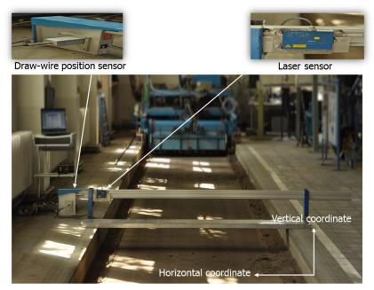
Figure 2: Laser scanner (© A. Al-Neama)
