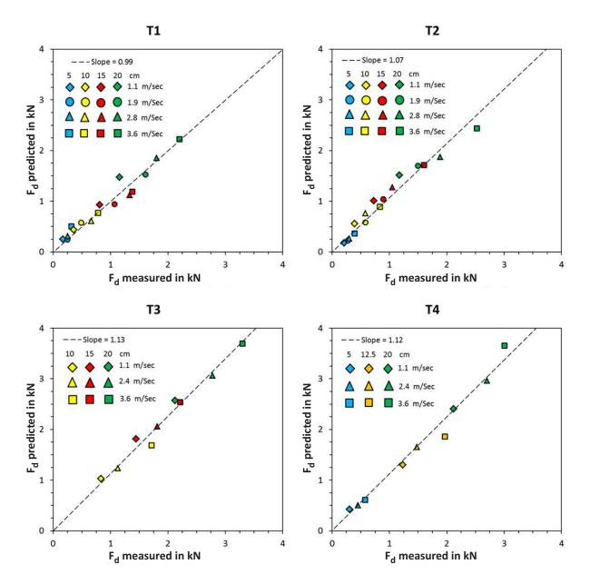
Figure 4: Correlation between measured  $F_d$  and predicted  $F_d$  for all measured tines in soil bin
