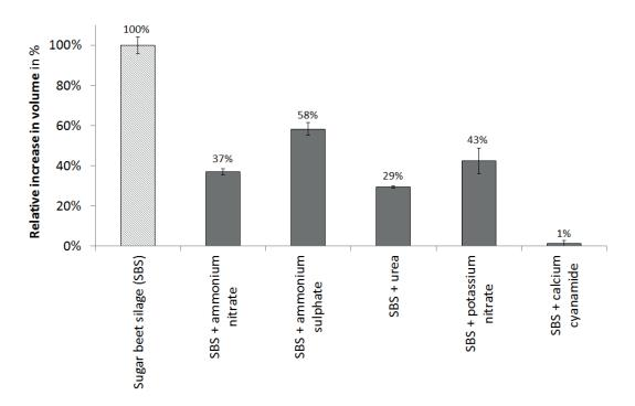
Figure 1: Relative increase in volume in foaming tests with the addition of 2.5 g/kg of nitrogen-containing compounds
