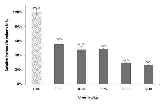
Figure 2: Relative increase in volume in foaming tests with 20 g/kg of SBS and 0 to 5 g/kg of urea
