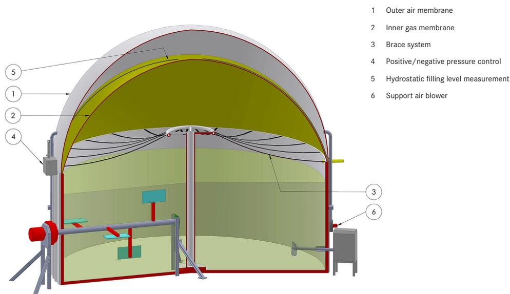
Figure 6: Structure continuous stirred-tank reactor (CSTR) with integrated double membrane gas storage, source: adapted from (Liebetrau et al. 2015)
