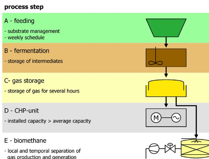
Figure 1: Approaches for a flexible operation of a biogas plant referring to the process chain, source: own diagram, based on ORTWEIN et al. (2014)
