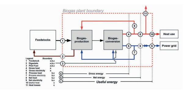
Figure 1: The assessment boundaries of the biogas process for assessing the gross, net and useful energy.
