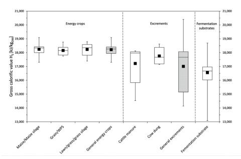
Figure 4: Ranges of variation, median values (line in the box), and averages (black dot) of the gross calorific values of dry matter.
