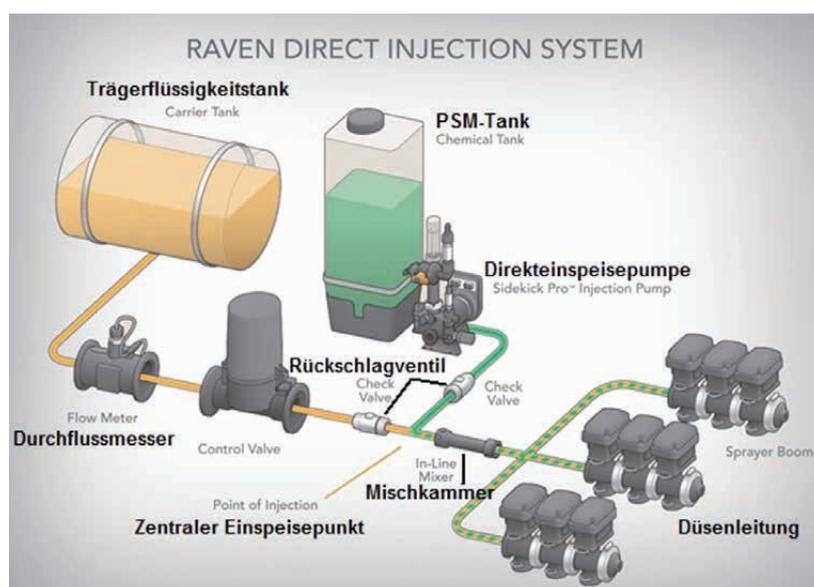
Figure 3: Diagram of Raven direct injection, altered (RAVEN 2015b)
