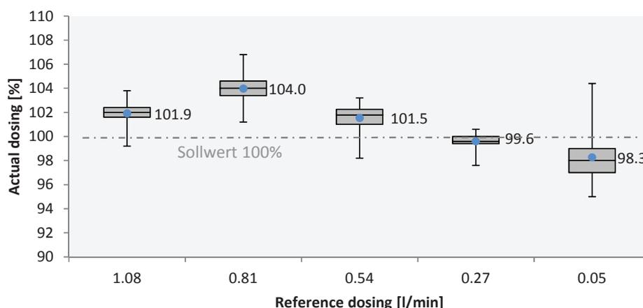
Figure 8: Dosing precision at different outputs for the small pump with a range of 0.03–1.18 l/min (n = 180)
