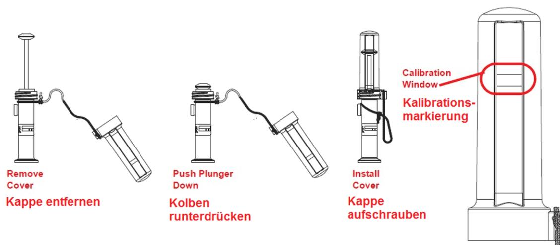
Figure 6: Calibrating the direct injection pump (RAVEN 2015a)
