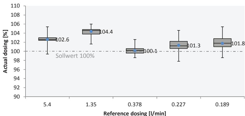
Figure 9: Dosing precision at different outputs for the large pump with a range of 0.15–5.9 l/min (n = 180)
