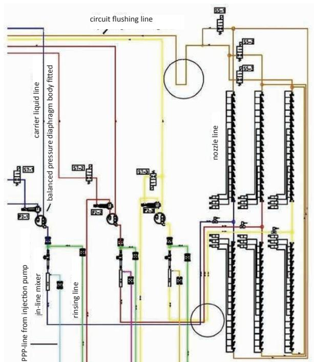
Figure 7: Section of fluid circuitry diagram from the prototype with three nozzle lines, altered (DAMMANN 2013)
