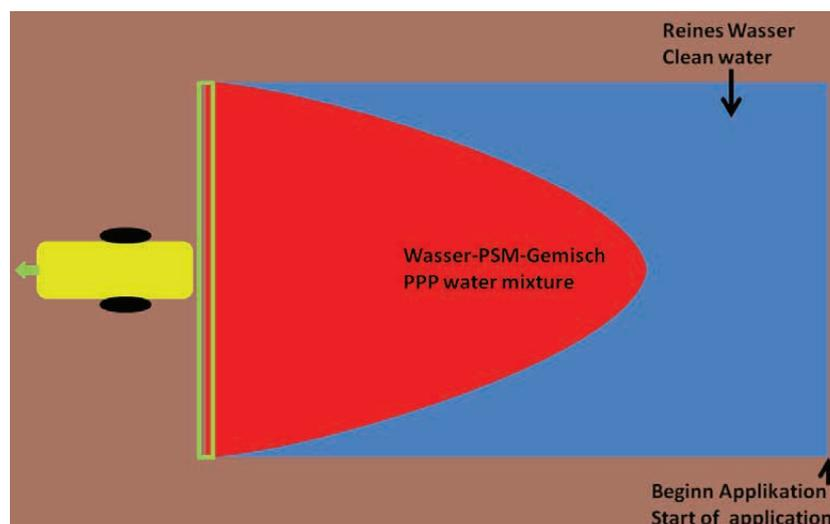
Figure 1: Diagram of the butterfly effect created through direct injection of spray material without preloading
