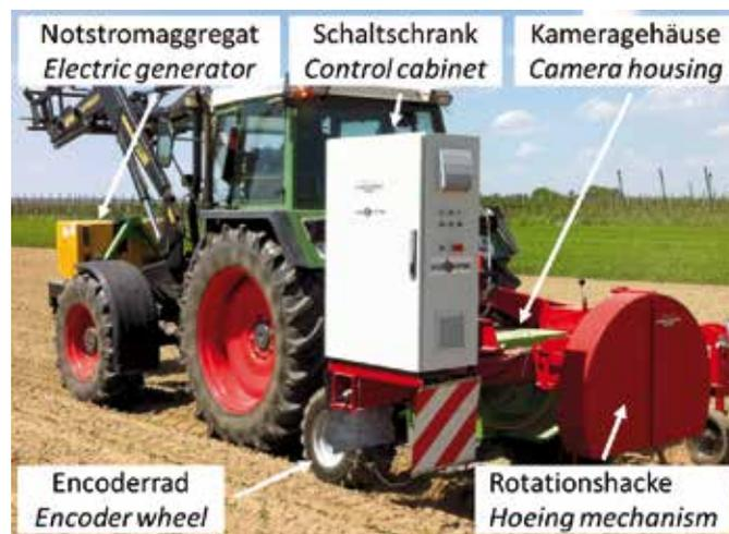
Test machine on a conventional tractor (Photo: Müter)
