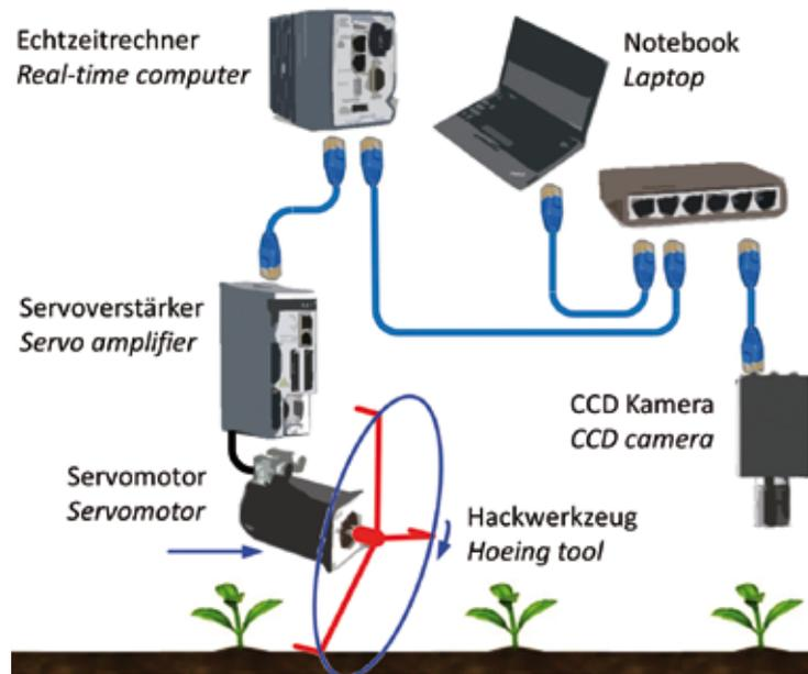
Basic setup of the test device. As a link between camera and servomotor, a real-time processor calculates new setpoints for the motor position.
