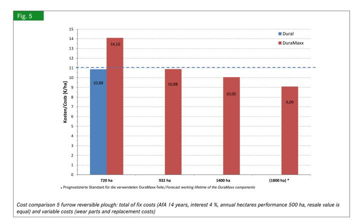
is greatly reduced by reducing the number of bolts required for attaching wearing components onto the frame. The cost comparison shows that the new material DuraMaxx already works out cheaper than the standard material Dural after 932 ha.
