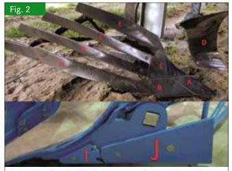
Description of the individual components of a plough bottom in the test (Photo: Reckleben)
