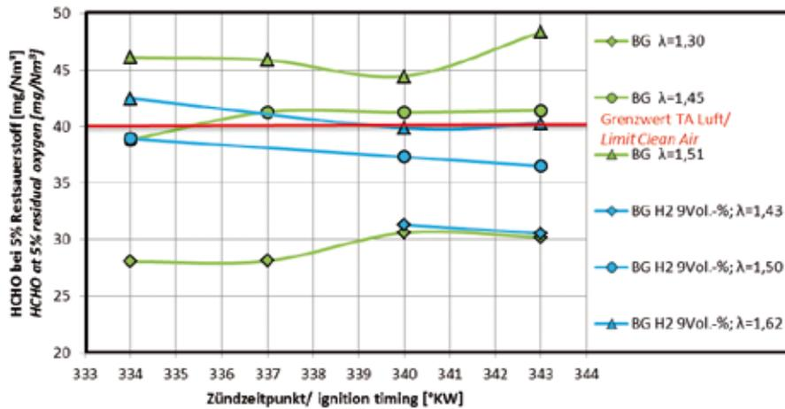
H<sub>2</sub> / Influence of ignition timing on the HCHO-emission of BG 50/50 with 0 and 9 vol.-% H<sub>2</sub> [4]
