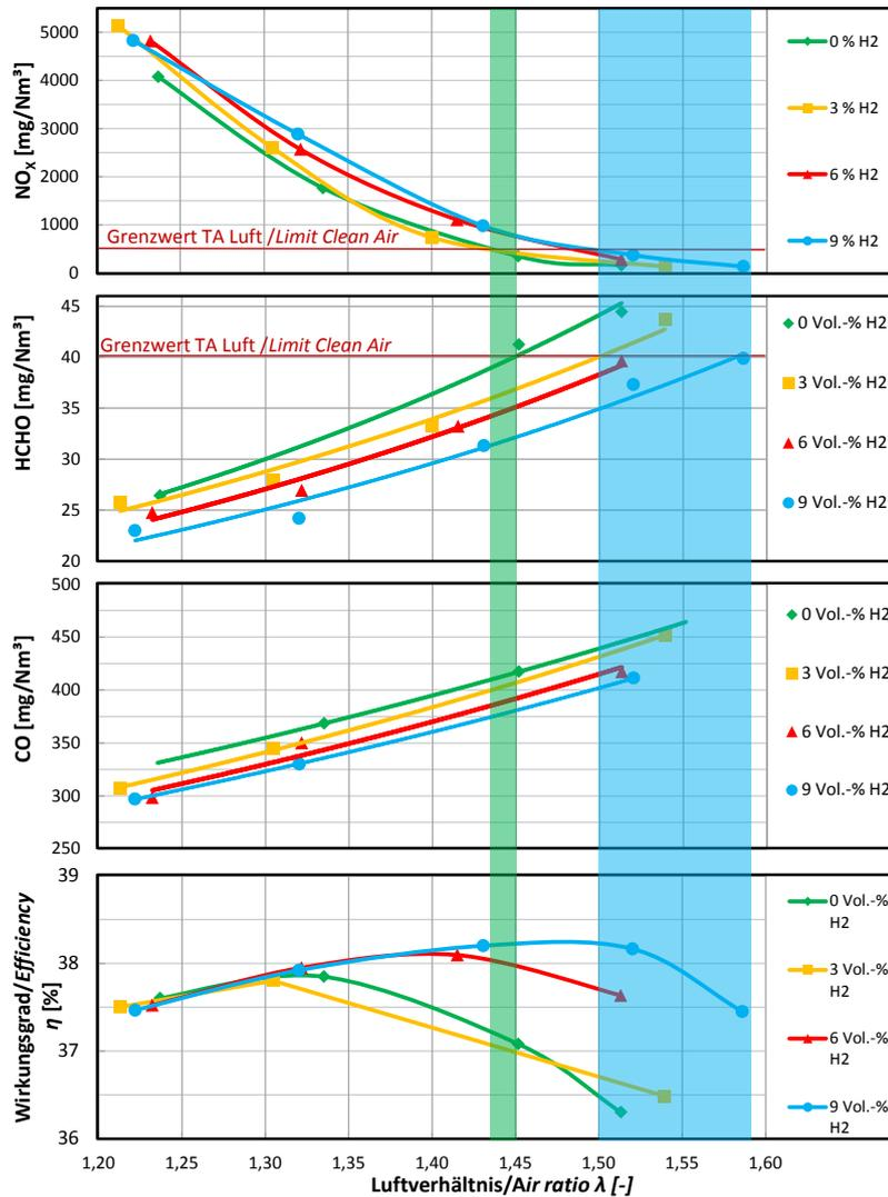
Influence of the hydrogen concentration and the air ratio on the efficiency and the exhaust emissions (NO<sub>x</sub>, HCHO, CO) at BG 50/50 [4]
