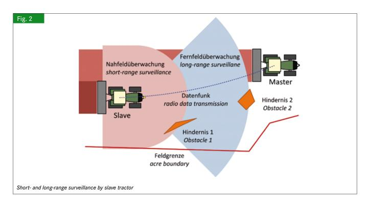
Once detected, obstacles are being tracked and stored in a local ambient map until they have been passed safely. The life cycle of an obstacle is protocolled from its time of detection (time of birth) including all interactions with the driver and other system modules. Thereby the system behavior can be retraced afterwards.
