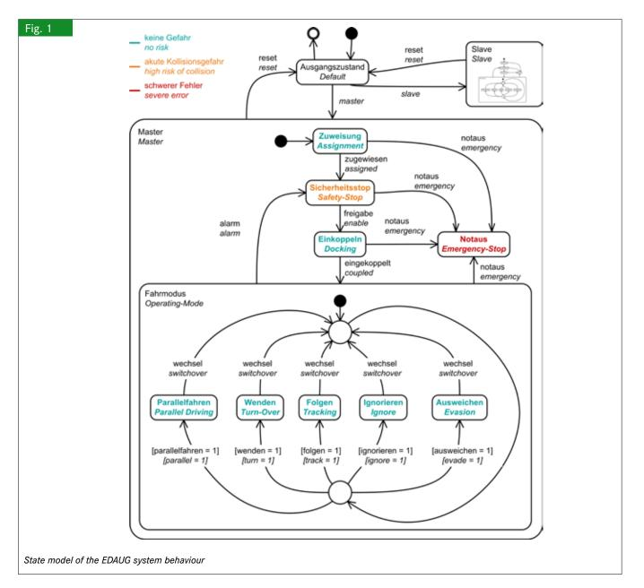
sibly evolve on a new path. If an obstacle warning (see safety concept) occurs, the driver is in charge to manually activate the Evasion mode.
