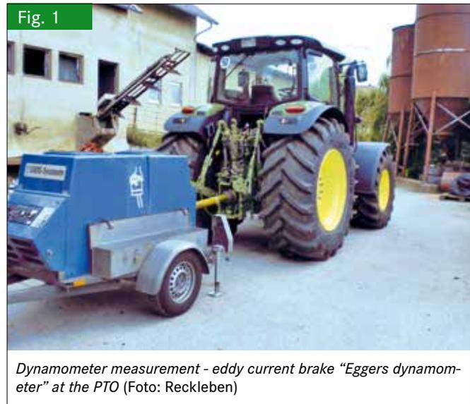
*Dynamometer measurement - eddy current brake "Eggers dynamometer" at the PTO (Foto: Reckleben)*
