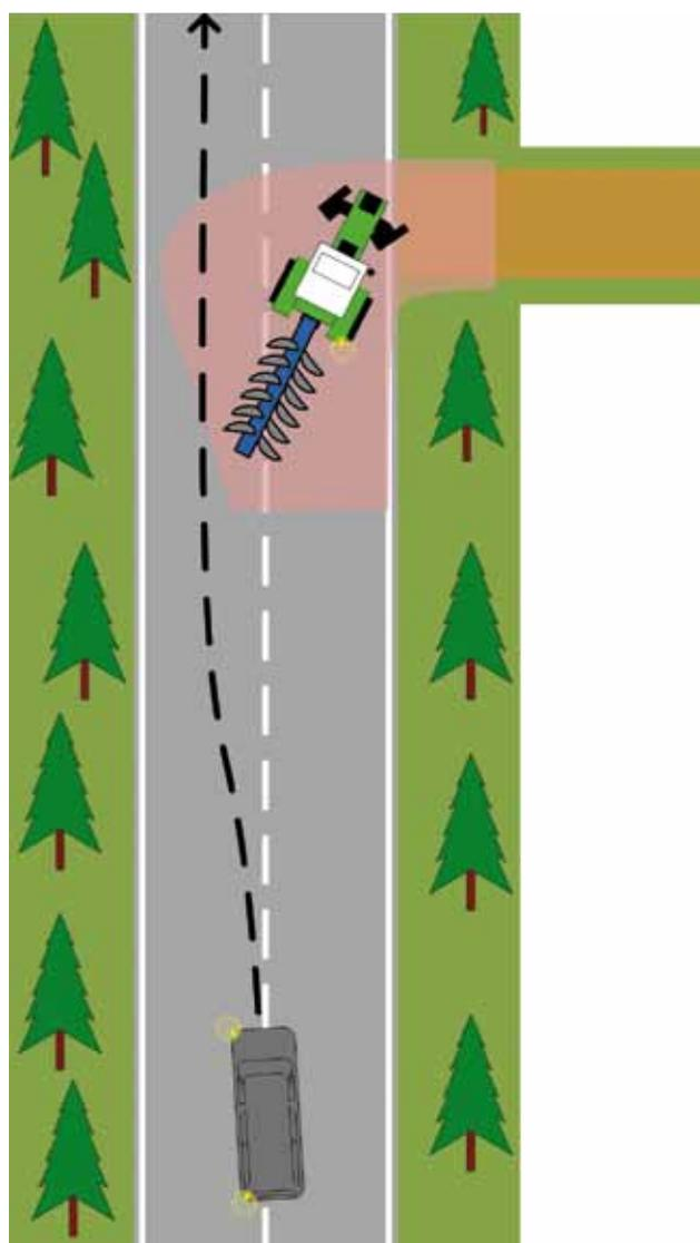
Turning tractor with swinging out implement, overtaking car and marked danger zone
