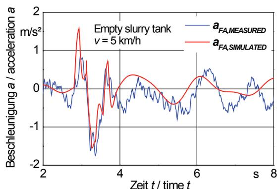
Front axis acceleration while driving over an obstacle, measured and simulated
