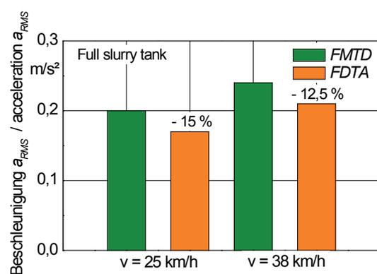
Driver seat acceleration for passive control while driving on the road
