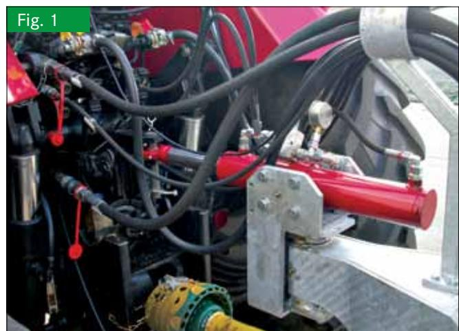
Top cylinder installed above the connection between tractor and trailer
