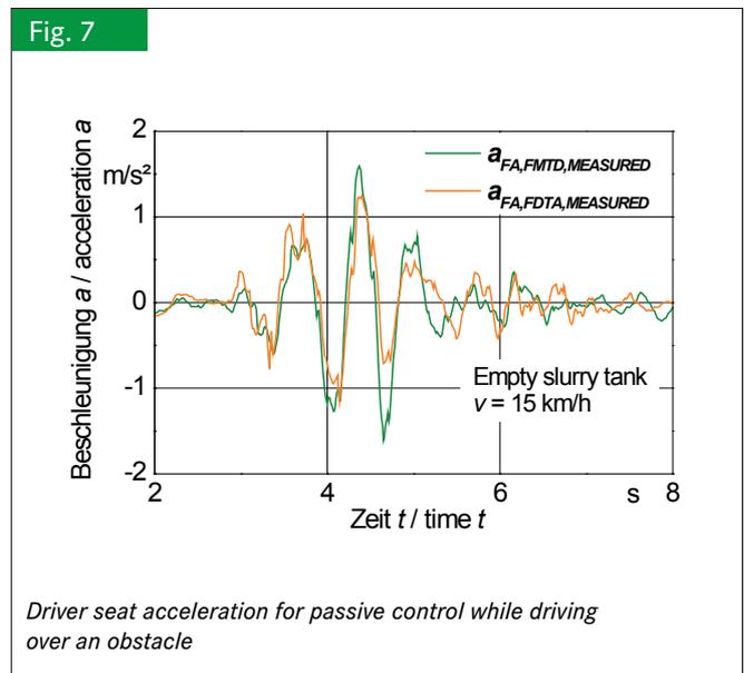
Driver seat acceleration for passive control while driving over an obstacle
