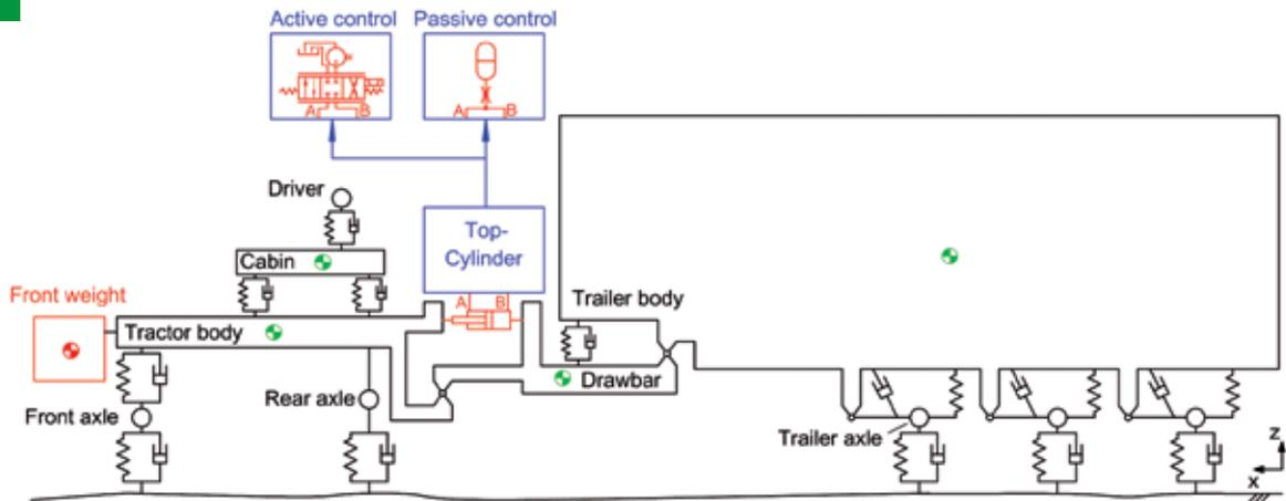
Simplified, two-dimensional vibration model of a tractor-trailer combination with fixed drawbar and top cylinder
