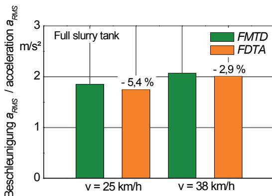
Front axis acceleration for passive control while driving on the road
