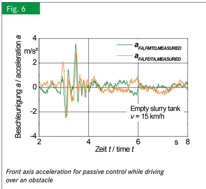
Front axis acceleration for passive control while driving over an obstacle
