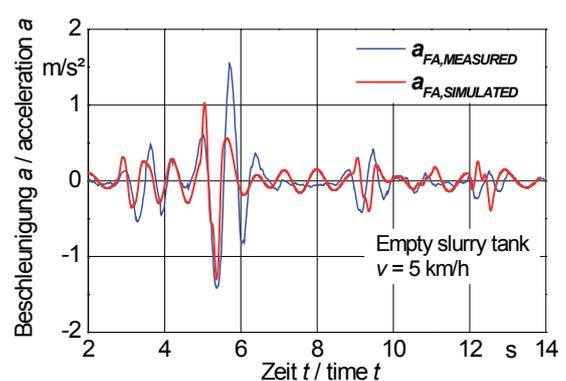
Driver seat acceleration while driving over an obstacle, measured and simulated
