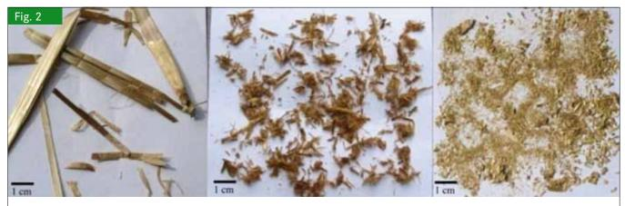
Untreated (left), wet extruded (middle), and dry extruded straw (right)
