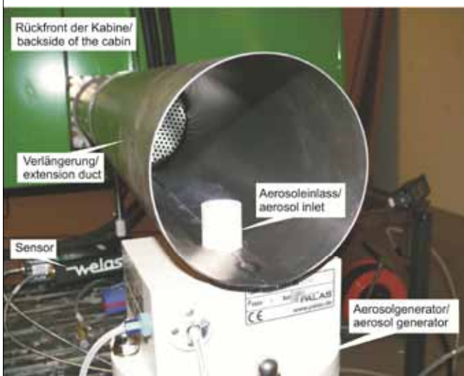
Test assembly to measure the protection efficiency according to the aerosol test
