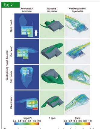
The rows show the ammonia concentration in an horizontal cut 0.5 m above floor, the ammonia cloud of 1 ppm leaving the stable and the path lines of fluid parcels of air at a wind velocity of 1 m/s; the columns show the influence of different directions of incoming wind
