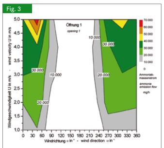
Example for the emission behaviour of the opening 1. White marked are the areas without emission and in colour shades the areas of emissions
