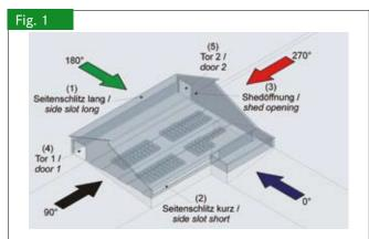
Planned box stable with openings at th end of fhe feed alley (4), (5), in the sidewalls (1), (2) and in the roof (3). The arrows show the direction of the incoming wind
