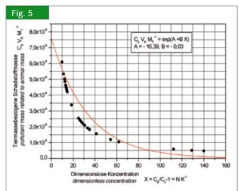
Graphical representation of the substitution function, which covers all stable openings for the mass outlet and is used as avarage function
