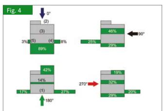
In dependency on the wind direction the incoming wind blows the stable air loaded with ammonia through the openings with different rates, e.g. by the wind incidence from 180° (south) through the opening (5) with 17%, through the opening (4) with 27%, through the opening (2) with 42% and through the opening (3) with 14%
