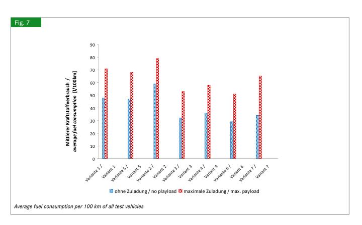
the same section. The average fuel consumption of semi-trailer truck 1 while driving fully loaded (40 t gross vehicle weight) is 51 L/100 km and 62 L/100 km for semi-trailer truck 2. The difference in fuel consumption seems to be higher, when driving loaded trucks. In this case, the additional fuel-consumption is a result of a combination of technique and driving style.
