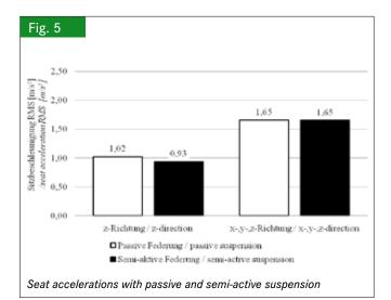
evident. Intelligent control concepts can help to improve driving comfort. To use the full potential of the semi-active suspension and increase driving comfort as well as driving safety further research will be done at the TU Berlin.
