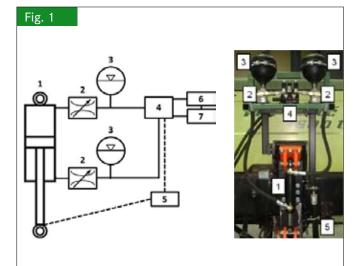
Installed hydropneumatic suspension system
