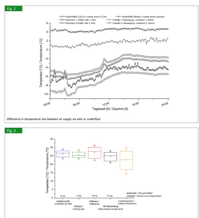
Range of temperatures of inlet air and indoor air
