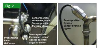
NIR sensor in a bypass, two other sensors in front of the same digester
