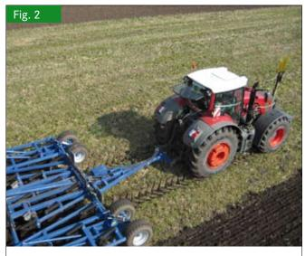
Fig. 2: Adjusted tire inflation pressure (pictured: 0.6 bars) results in less soil deformation and more driver comfort
