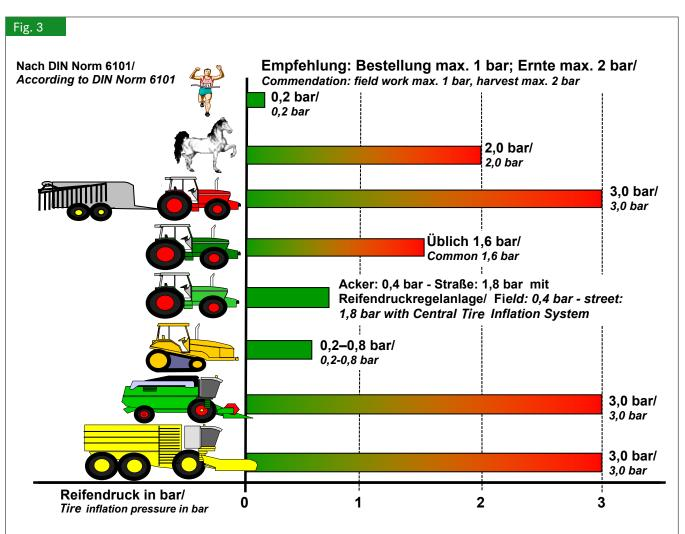
Fig. 3: 1 bar for seeding and 2 bar tire inflation pressure for harvesting should be the maximum tire pressure
