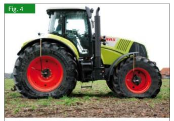
Fig. 4: Backfitted "Strotmann" Central Tire Inflation System (CTIS) (appr. 2.500 €) with air hoses above the fenders. System functions are centrally managed with the StG-Terminal
