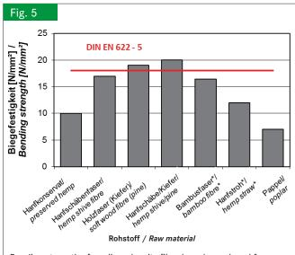
Bending strength of medium density fibre boards produced from different raw material (\*density 550 kg/m<sup>3</sup>, all other densities 600 kg/m<sup>3</sup>)
