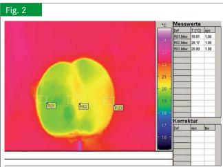
Temperature distribution on the surface of a peach during drying off surface moisture using infrared thermography, measuring points R01, R02 und R03
