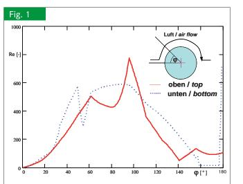
Measured proceed of Reynold's number of the air flow along a peach fruit surface; solid line: along upper half, dashed line: along lower half of fruit
