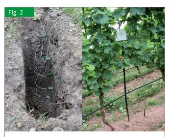
Soil moisture sensors (left) and wireless node for data transfer of soil moisture data (right)
