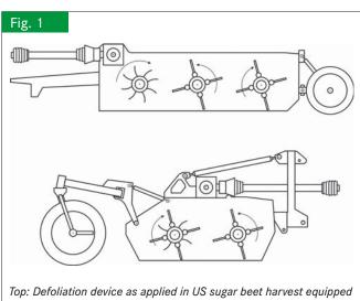
with 3 shafts as trailed implement. Bottom: Unit for tractor front mounting or as header of six row harvester
