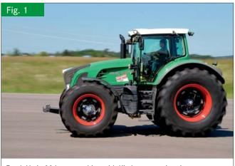
Fendt Vario 936 test machine with Kistler measuring rims
