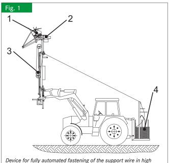
trellis of hop. 1: positioning unit, 2: wire tying unit, 3: intermediate storage of the wire, 4: wire coil
