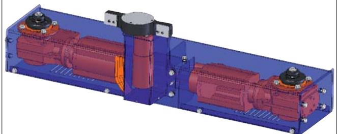
Transparent view of the electrical disc/agitator drive of a fertilizer spreader
