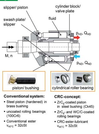
Hydraulic displacement pump; conventional and CRC-concept
