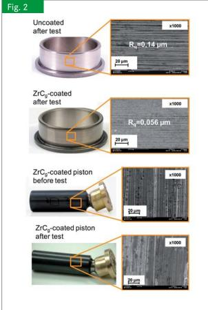
Rolling bearings after test (top), pistons before and after test (bot-tom)
