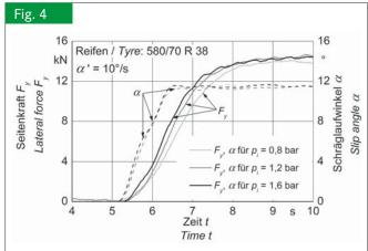
Measured slip angle and the corresponding lateral forces for a 580/70 R 38 tyre at different tyre pressures and a stationary wheel load of 20 kN
