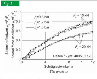
*Quasi steady-state lateral force coefficient at different stationary loads and tyre pressures for a 480/70 R 28 tyre on asphalt*
