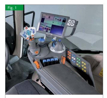
Armrest with the new Fendt Varioterminal 10.4" as an example for a manipulation with touchscreen and navigation buttons. Photo: Fendt
