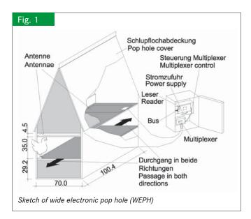
a maximum time of 500 ms. This results in a total duration of between 100 ms and 1 s for a whole reading cycle at both antennae.
