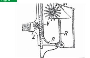
With the 1885 Schloer fertiliser spreader, the hoppers were moved to the spreading mechanism via rack and pinion gearing
