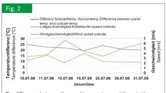
The difference between the panel temperature and the outside temperature shows a good correlation with the wind speed and the air speed in the collector
