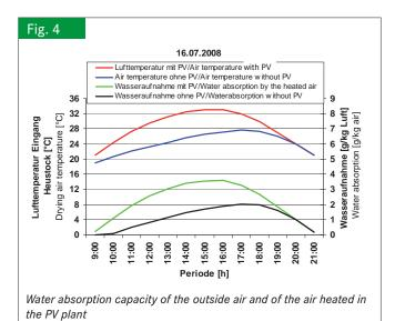
When using the heated air of the photovoltaic plant for drying hay, the drying period can be halved.
