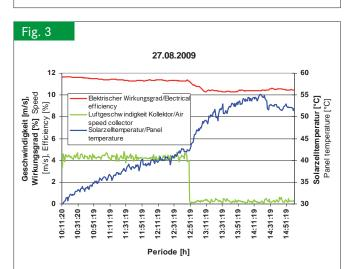
Switching off the fan leads to a rapid increase in the panel temperature from  $42^{\circ}$ C to  $55^{\circ}$ C and a decrease in electrical efficiency from 11.2 to 10.4%
