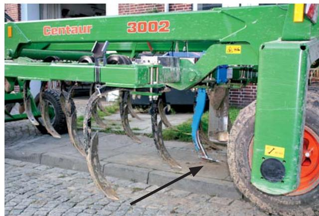
Impedance sensor for soil water mounted to the front bar of the cultivator
