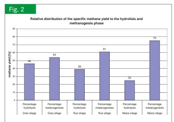
Relative distribution of the specific methane yield of the various stages (hydrolysis and methanogenesis) in the two-phase anaerobic digestion of various renewable resources
