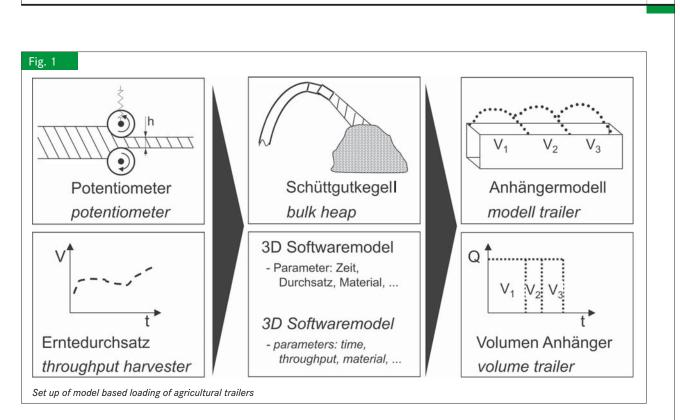
divided into several discrete volume spaces. By generating and achieving loading points the discrete spaces are to be filled up to the maximum load of the trailer. Regarding the throughput and the effective loading position a software model estimates the loading state inside the trailer, until it is filled at maximum rate. **Figure 1** depicts the set up principle.
