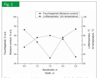
Moisture content and air temperature across the belt width in the middle of the first band
