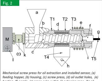
feeding hopper, (b) housing, (c) screw press, (d) oil outlet holes, (e) heating, (f) nozzle, (g) press cake outlet, (i) cohesion zone, (h) oil collector, (k) coupling, (l) speed alternator, (M) motor, (T1-T5) temperature sensors, (T5) temperature sensor (IR), ( $\Omega$ ) rotational speed
