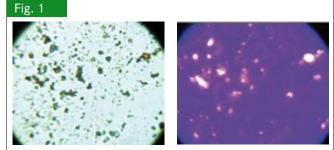
Sample, illuminated with transmitted white light (left) respectively incident ultraviolet light (right)
