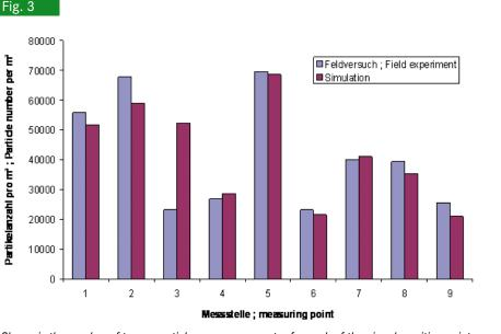
Shown is the number of tracer particles per square meter for each of the nine deposition points. Experimental data is shown in red, while blue shows the simulation results.
