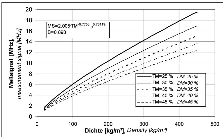
Fig. 1: Effect of the parameters density  $\rho$  and dry matter content DM on the measuring signal MS of a microwave sensor during measuring the density of eleven silage samples (forage maize and gras)
