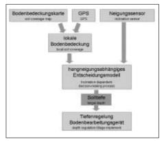
*Fig. 1: Decision making and control of tillage depth*
