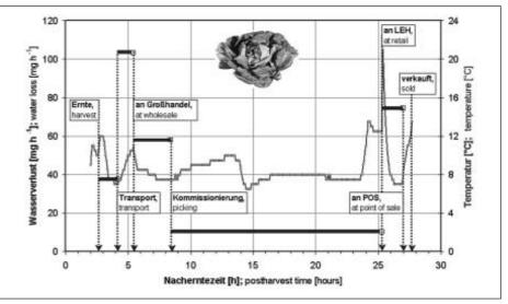
Fig. 2: Control of the climatic loads of lettuce in the postharvest chain by means of temperature devices and evaporation spheres
