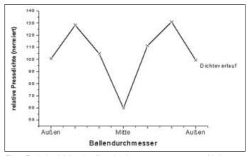
Fig. 3: Typical axial density allocation for a constant-room round bale (straw)
