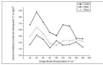
*Fig. 2: Density allocation in three levels of a straw square bale*
